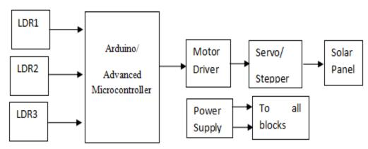
Figure 4: Block diagram of solar tracking system
