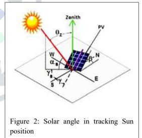
referenced by A. R. Amelia et al [14]. They mention that, altitude(elevation) and azimuth is most important angle in determining the position of sun. Solar irradiance can be obtained by measuring the power of the light sources or the luminous flux. The elevation angle ( $\alpha$ s) and zenith angles( $\theta$ z) have close definition is to the declination angle. Declination angle ( $\delta$ ) is the angle between equator and a line drawn from the centre of the sun to the centre of
