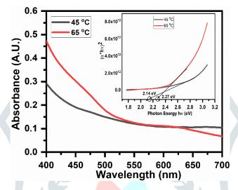
**Figure 5:** The UV-Visible spectrum of 45 °C and 65 °C temperature thin film prepared PbS samples. **IV. Conclusion:**
