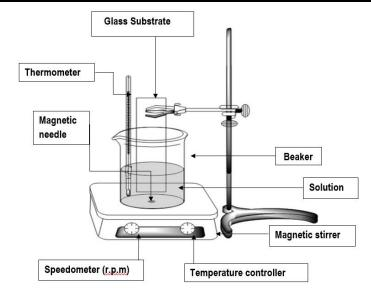
Figure 2: Schematic layout of chemical bath deposition method.
