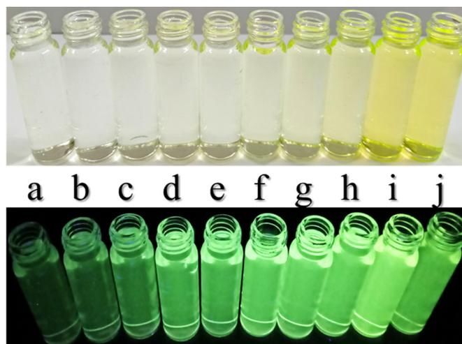
Fig. 9. Digital images under UV lamp and visible light; a-FNH in acetone, b-FNHNPs, c-FNHNPs + 2 μg/mL Cu<sup>2+</sup>, d-FNHNPs + 4 μg/mL Cu<sup>2+</sup>, e-FNHNPs + 8 μg/mL Cu<sup>2+</sup>, f-FNHNPs + 12 μg/mL Cu<sup>2+</sup>, g-FNHNPs + 16 μg/mL Cu<sup>2+</sup>, h-FNHNPs + 20 μg/mL Cu<sup>2+</sup>, i-FNHNPs + 24 μg/mL Cu<sup>2+</sup>, j-FNHNPs + 28 μg/mL Cu<sup>2+</sup>.
