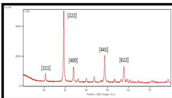
Fig. 4 XRD for 4 %  $Eu^{3+}$  doped  $Y_2O_3$  NPs
