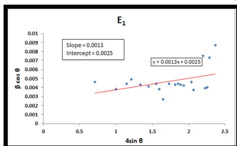
**Fig. 5 The W-H plot for 1 % Eu:  $Y_2O_3$**
