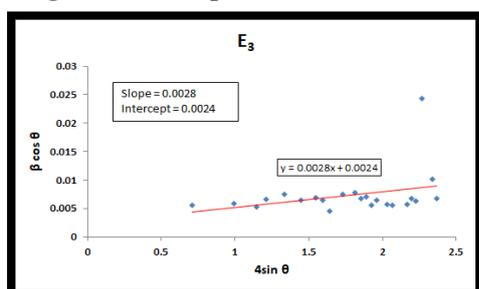
**Fig. 7 The W-H plot for 3 % Eu:  $Y_2O_3$**
