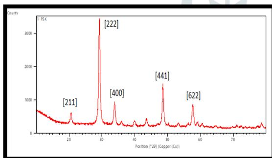
Fig. 1 XRD for 1 %  $Eu^{3+}$  doped  $Y_2O_3$  NPs
