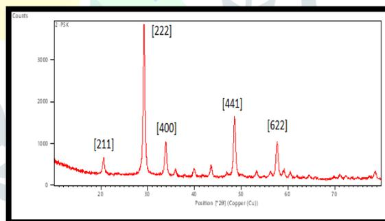
Fig. 2 XRD for 2 %  $Eu^{3+}$  doped  $Y_2O_3$  NPs
