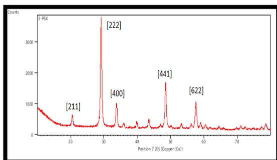
Fig. 3 XRD for 3 %  $Eu^{3+}$  doped  $Y_2O_3$  NPs
