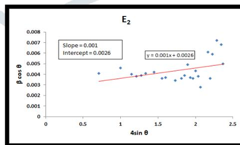
**Fig. 6 The W-H plot for 2 % Eu:  $Y_2O_3$**
