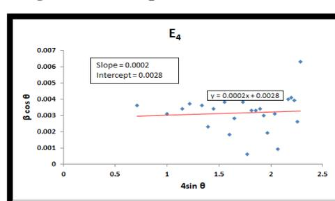
**Fig. 8 The W-H plot for 4 % Eu:  $Y_2O_3$**
