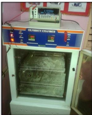
Figure 3: Experimental arrangement for humidity dependent resistance measurement.
