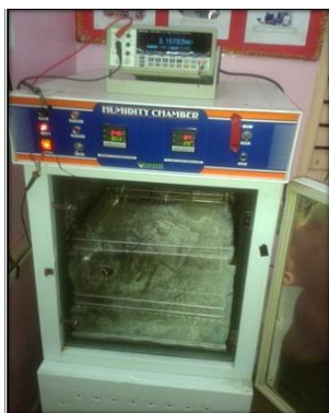
Figure 3: Experimental arrangement for humidity dependent resistance measurement.
