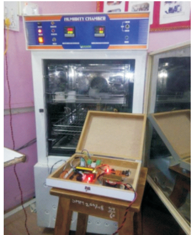
Figure 11. Experimental Setup Calibration of System for Humidity
