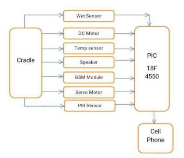
**Working-** When child is ready for sleep in cradle various sensor like noise sensor, PIR, wet sensor ,temperature sensor are used to monitor the child .firstly if the baby is in cradle the system is activated. When baby is crying the noise sensor gets input and system activate the music through Speaker and swing cradle is performed. Swing of cradle is performed by servo motor and toy start rotating due to DC motor.
