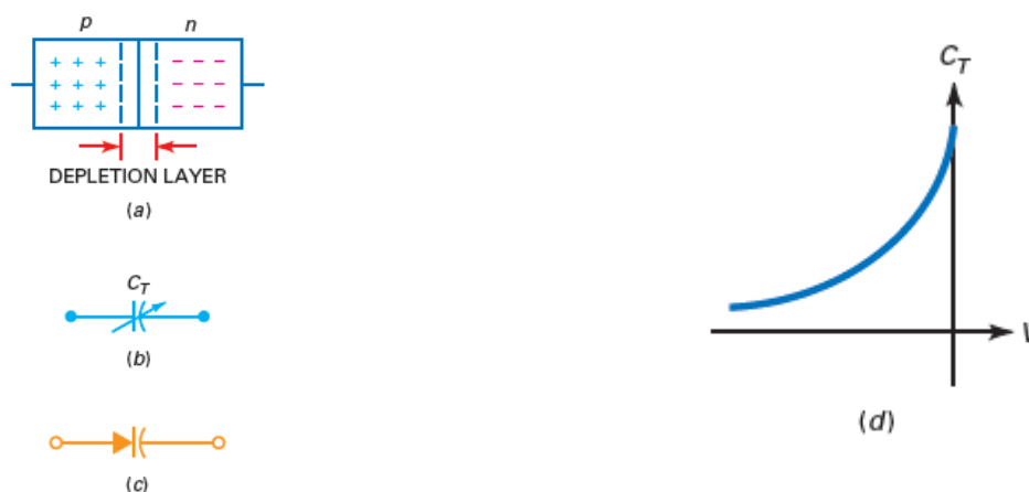
Fig5: Varactor.(a) Doped regions are like capacitor plates separated by a dielectric;(b) ac-equivalent circuit; (c) schematic symbol; (d) graph of capacitance versus reverse voltage
