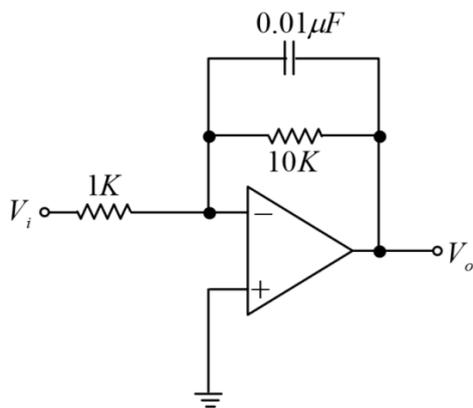
21) For this circuit the what is the frequency above which the gain will decrease by 20 dB per decade and At 2. 1kHz the value closed loop gain .
