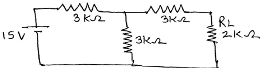
28. Determine Norton's equivalent circuit for the following network.
