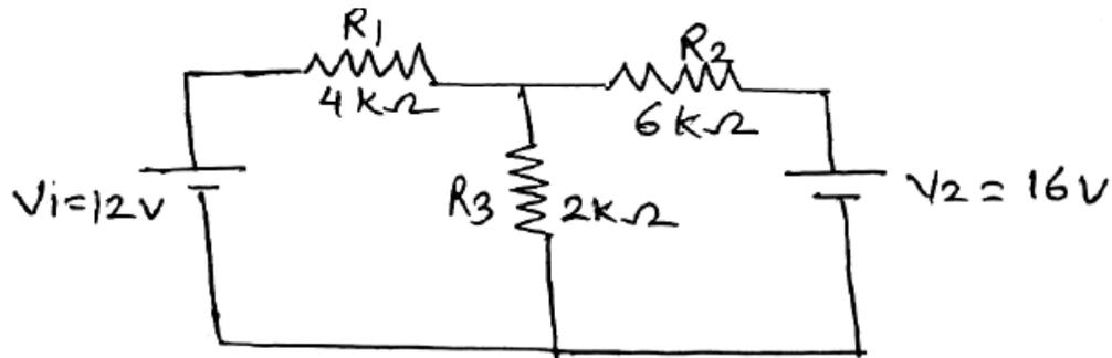
26. Determine Thevenin's equivalent circuit for the following network.
